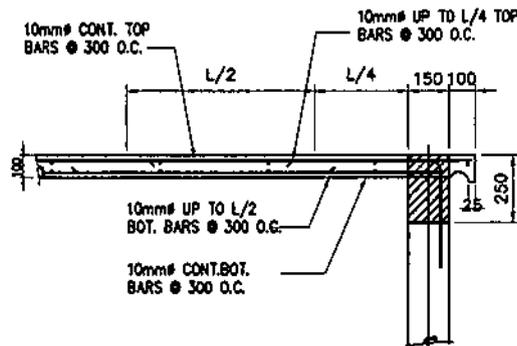
**ROOF SLAB REINFORCEMENT**
