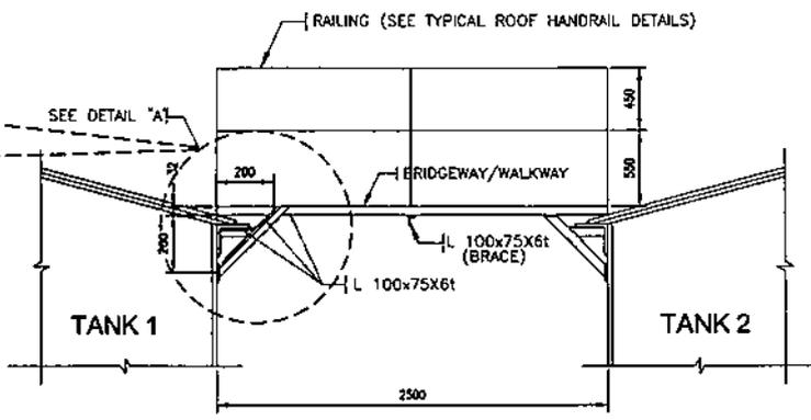
TYPICAL BRIDGE/WALKWAY FOR TWO (2) ADJACENT 60 CU. M. TANKS
